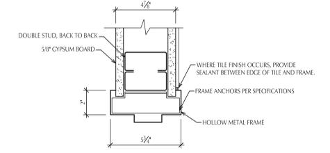
**Hollow Metal Door Frame Standard Detail**
