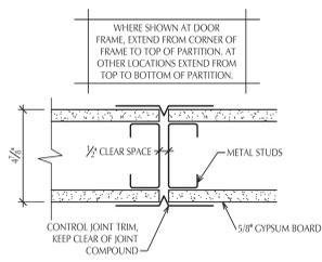
**Gypsum Board Partition Control Joint Detail**
