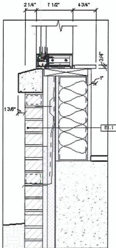
Window stools and wall cap at the stair rail walls are indicated in the drawings to be Solid Surface. Hanex as indicated appears to be a brand name. What solid surface product the Contractor submits is per the Contractor,
