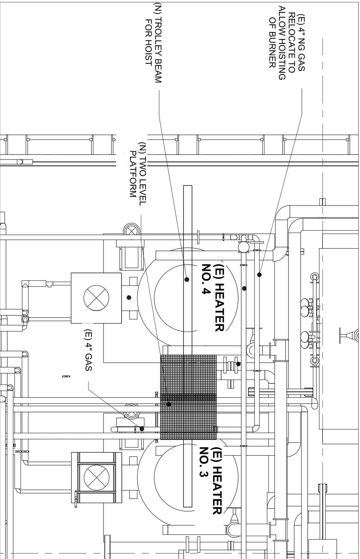
PROPOSED SOLUTION FOR CATWALK AND HOIST REQUIREMENT
