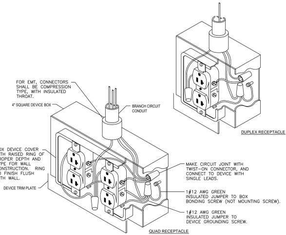
**11 DETAIL: TYPICAL RECEPTACLE WIRING DIAGRAM**
