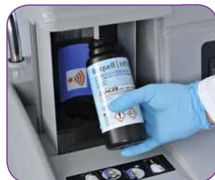
Image 3. Safe and secure bottle loading mechanism
