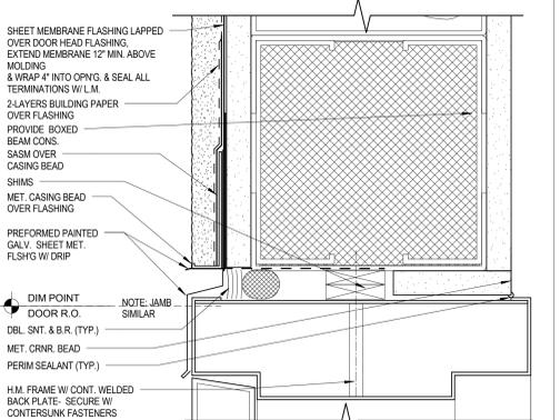
5 HOLLOW METAL DOOR FLASHING - HEAD
