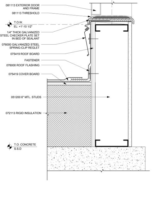
9 THRESHOLD AT LEVEL 2 EXTERIOR DOOR
