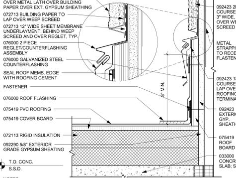
2 TYP. FLASHING AT STUCCO WALL
