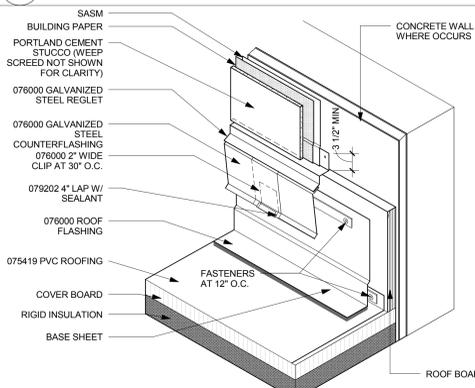
1 ROOF COUNTER FLASHING DETAIL
