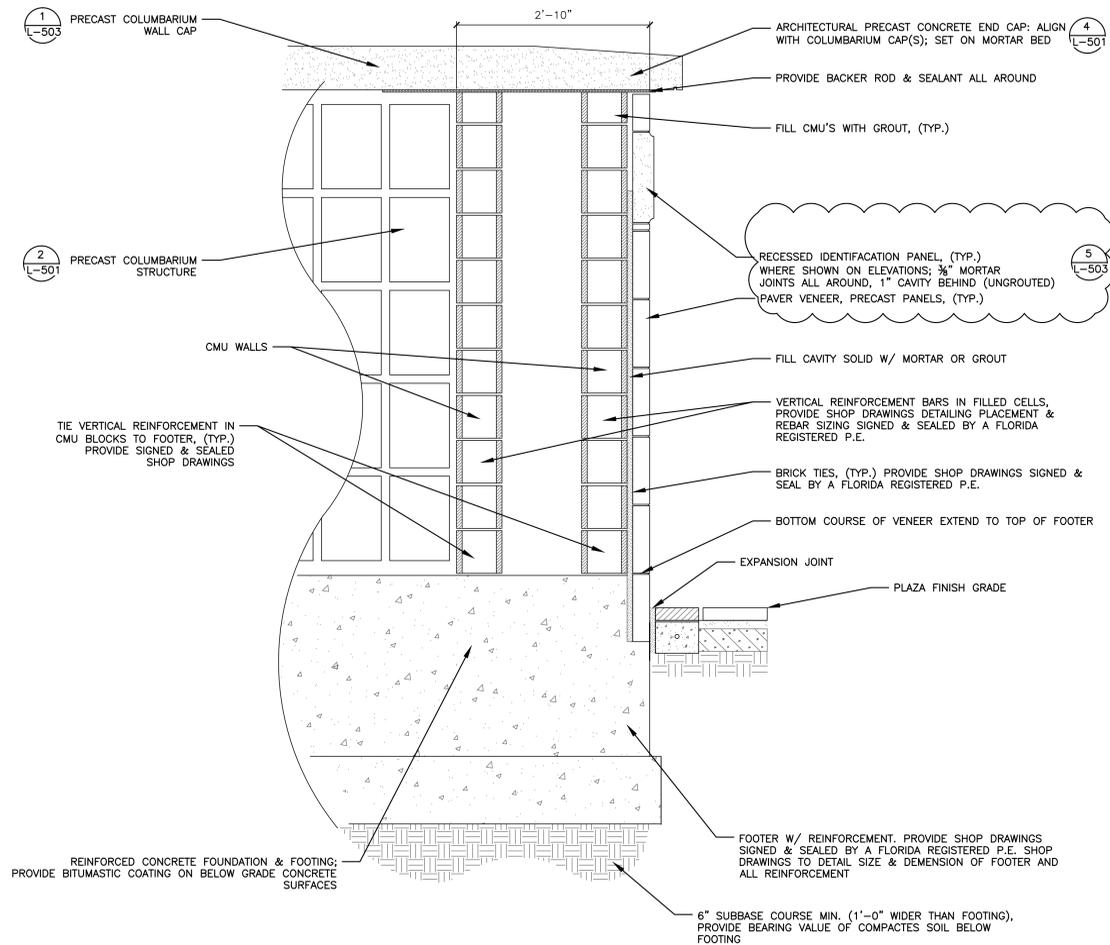
1 TYPICAL END WALL "PIER" - SECTION SIDE
