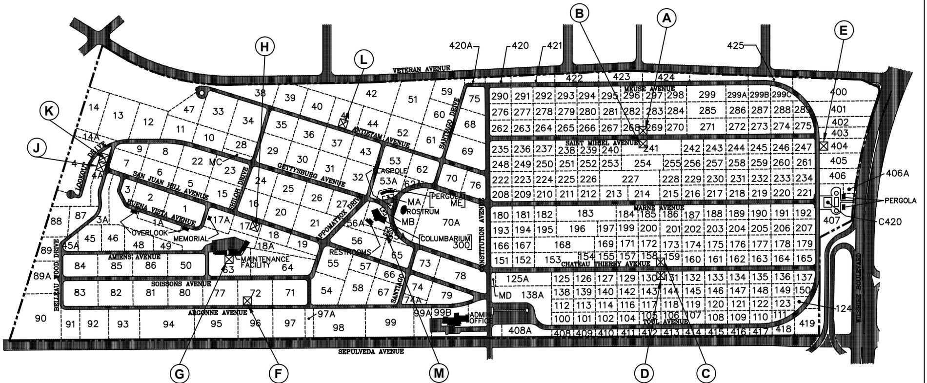
**MASTER VALVES TO BE REPLACED: A, D, E, F, G, L and M**
