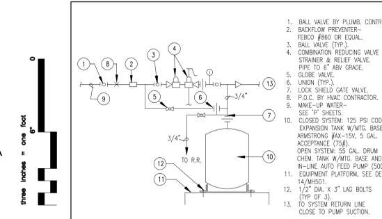
22 CW MAKE-UP AND TANK PIPING/ MTG. NTS
