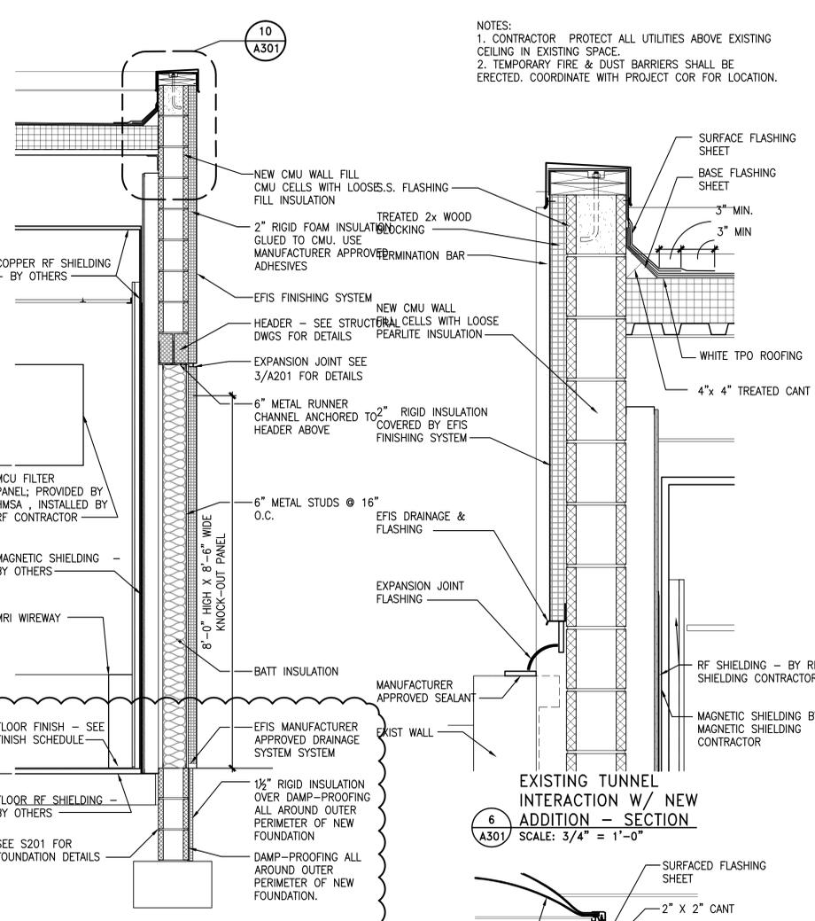
**6 EXISTING TUNNEL INTERACTION W/ NEW ADDITION - SECTION**
