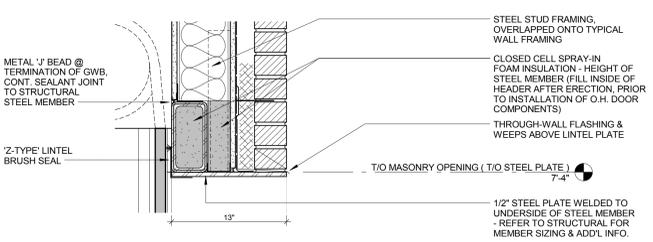
**6 SECTION DETAIL - OVERHEAD DOOR HEAD**
