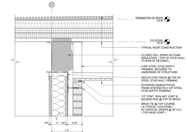
**5 DETAIL - TOP OF BRICK WALL @ UNDERSIDE OF ROOF**
