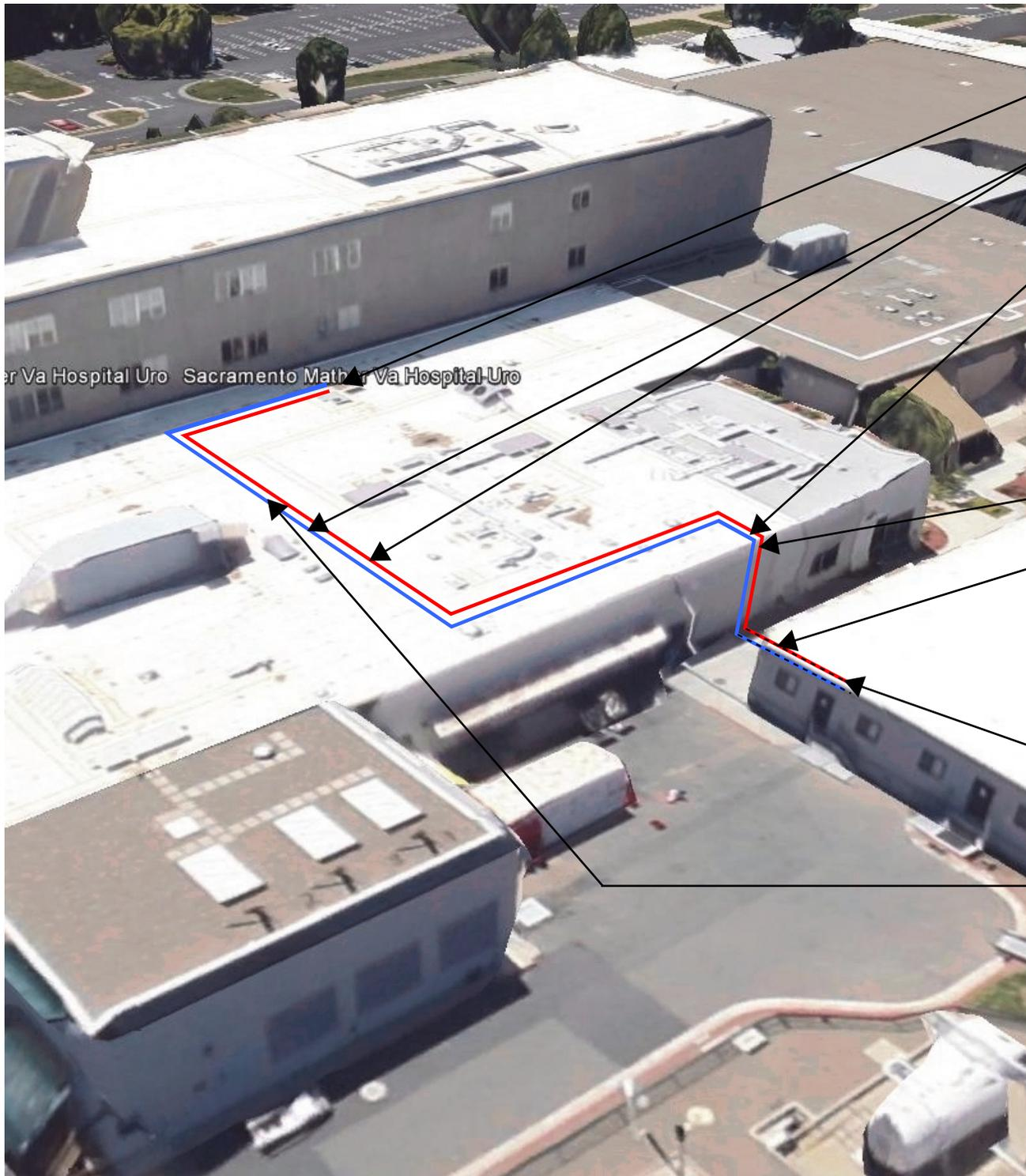
APPROXIMATELY 260 LINEAR FEET BETWEEN CONNECTION POINT AND PARAPET WALL
