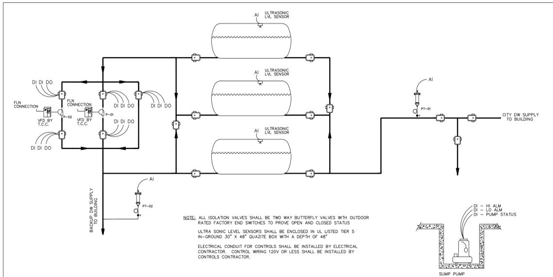
NOTE: ALL ISOLATION VALVES SHALL BE TWO WAY BUTTERFLY VALVES WITH OUTDOOR RATED FACTORY END SWITCHES TO PROVE OPEN AND CLOSED STATUS
