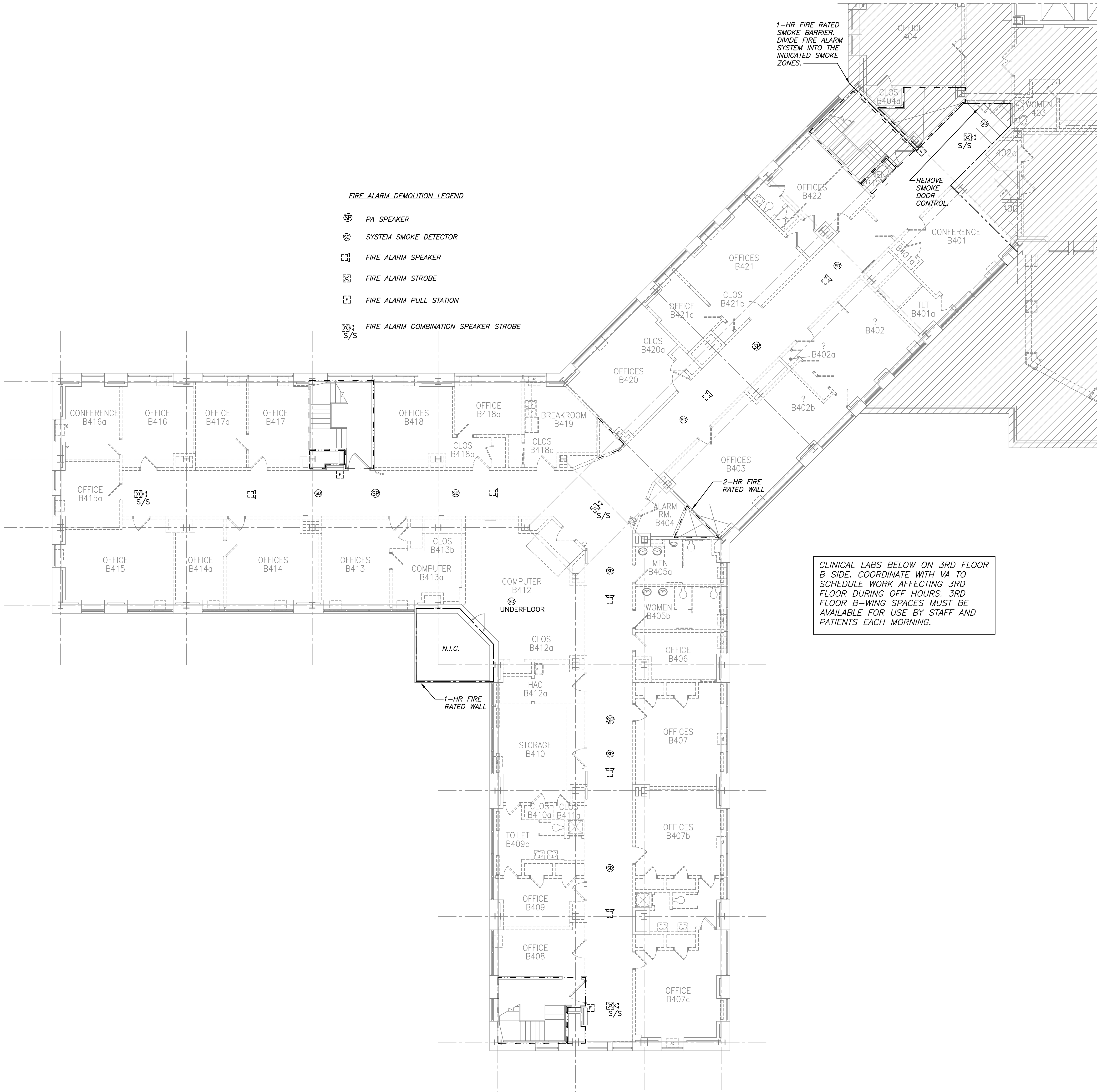
1 4TH FLOOR FIRE ALARM DEMOLITION PLAN - WING B F1.31 SCALE: 1/8" = 1'-0"
