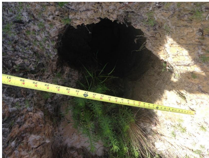
Photo 2: Top view of the existing sinkhole
