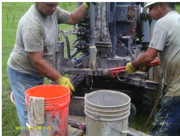
Photo 4: View of SPT drilling in progress
