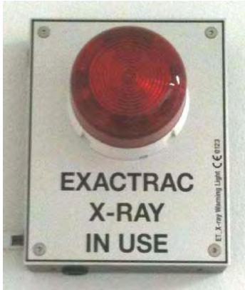
Figure 3-55 Wall Mounted ETX Warning Light
