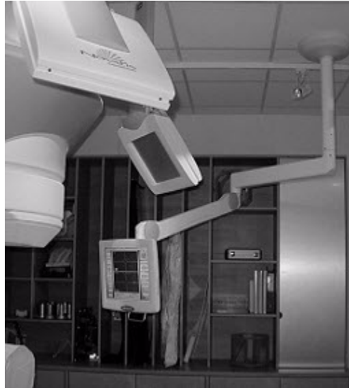
Figure 3-43 Ceiling Mounted In-Room Touch Screen Monitor
