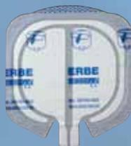
Because of its new shape the **NESSY  $\Omega$  Neutral Electrode** can be applied irrespective of direction. It practically precludes the troublesome “leading edge” effect, i.e. the development of high current densities at the electrode edges.
