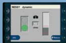
**NESSY** monitors the application of the patient plate, providing the user with information which is graphically displayed on the monitor
