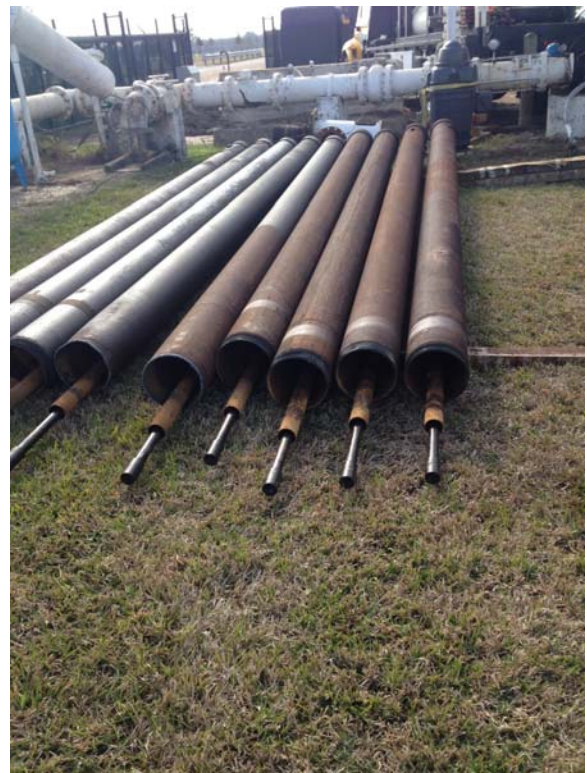
Figure 3: Pulled 10" pipe and tube shaft (currently still on site)
