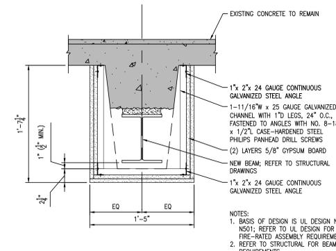
4 FIRE-RATED SOFFIT DETAIL
