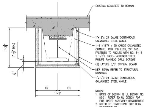
3 FIRE-RATED SOFFIT DETAIL
