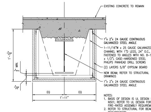
5 FIRE-RATED SOFFIT DETAIL
