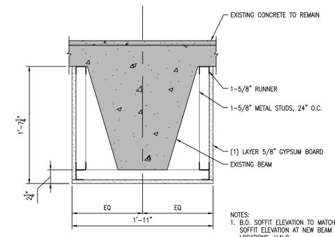
10 NON-RATED SOFFIT DETAIL
