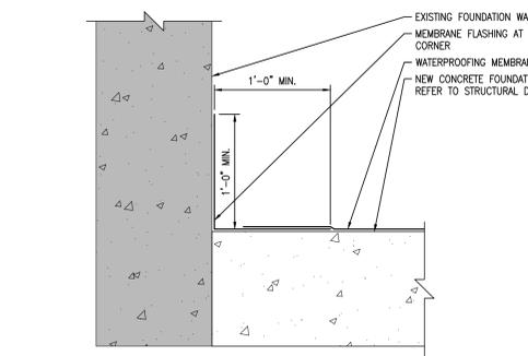
15 FOUNDATION WALL WATERPROOFING DETAIL
