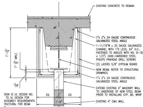
2 FIRE-RATED SOFFIT DETAIL
