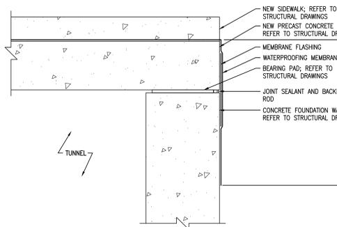
14 FOUNDATION WALL WATERPROOFING DETAIL
