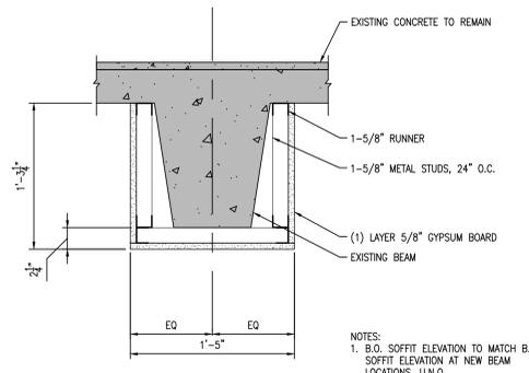
8 NON-RATED SOFFIT DETAIL
