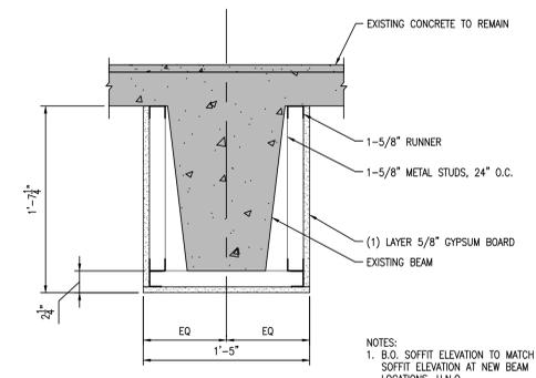
9 NON-RATED SOFFIT DETAIL
