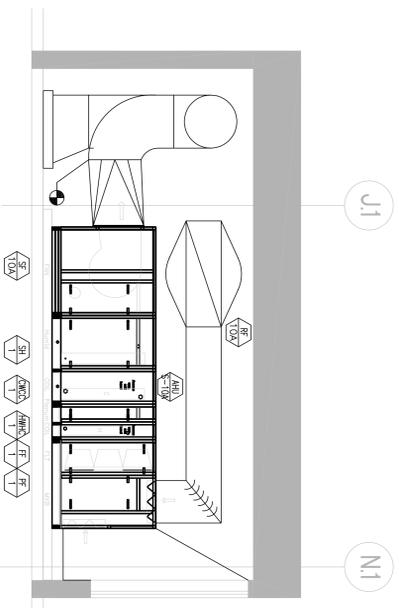
8 AIR HANDLER UNIT S-10A SECTION DETAIL
