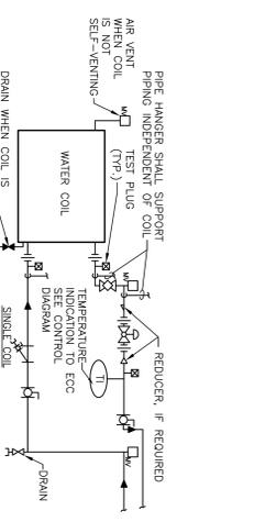
1 CHILLED WATER COIL - PIPING CONNECTIONS
