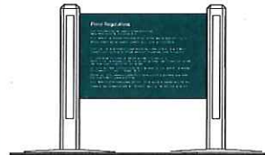
NC-01.01-c1&c2 2' x 3' panel 3'-6" tall Concrete post
