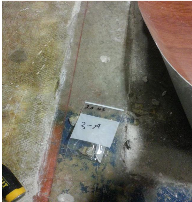
Homogeneous Area 3- Yellow Mastic
