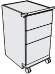
The handle shown in this location would not allow for the addition of an add-a-drawer and may not fit under the benches and/or tables in the project.
