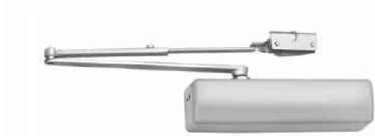
Parallel Arm Mounting DC6210, DC6410 Series Allows inside application of closer on out-swinging doors. Closer is mounted on the push side, with the arm almost parallel to the face of the door. Arm does not project from the opening.
