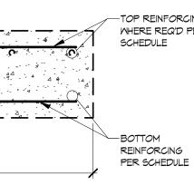
— BASE PLATE - SEE TYP. BASE -TOP REINFORCING WHERE REQ'D PER
