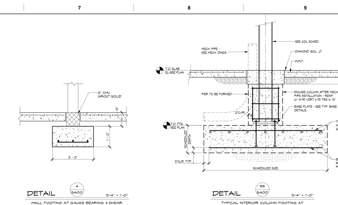
TYPICAL INTERIOR COLUMN FOOTING AT MECHANICAL PIPE
