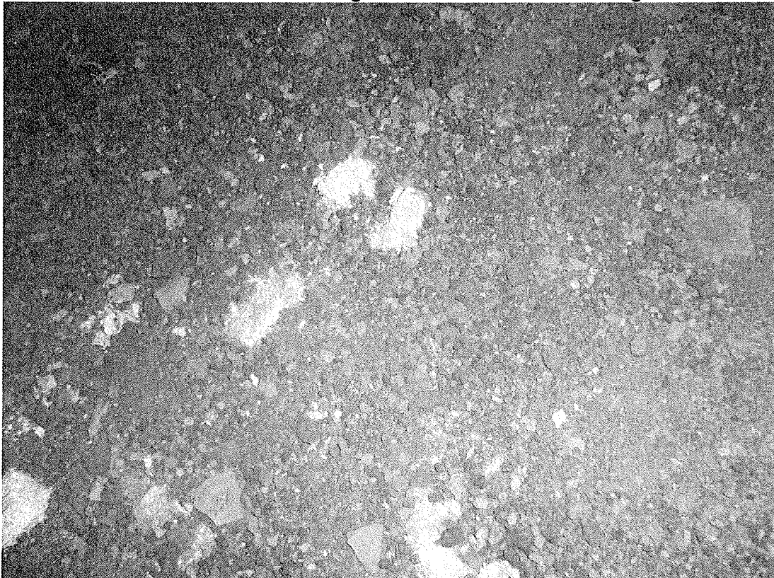
Asbestos pipe insulation debris in dirt of crawlspace – 20% Amosite
