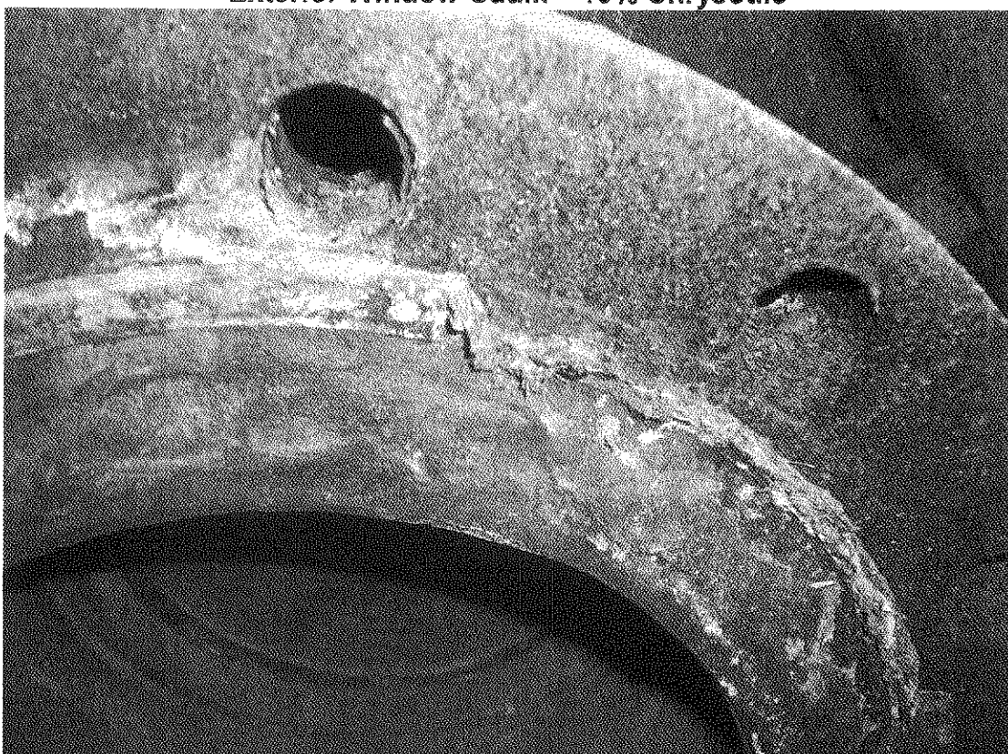
Steam Valve Gasket – 90% Chrysotile
