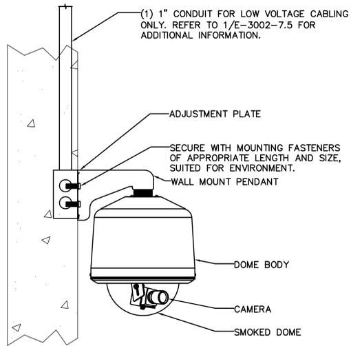
**5 EXTERIOR FIXED CAMERA WALL MOUNTING DETAIL**
