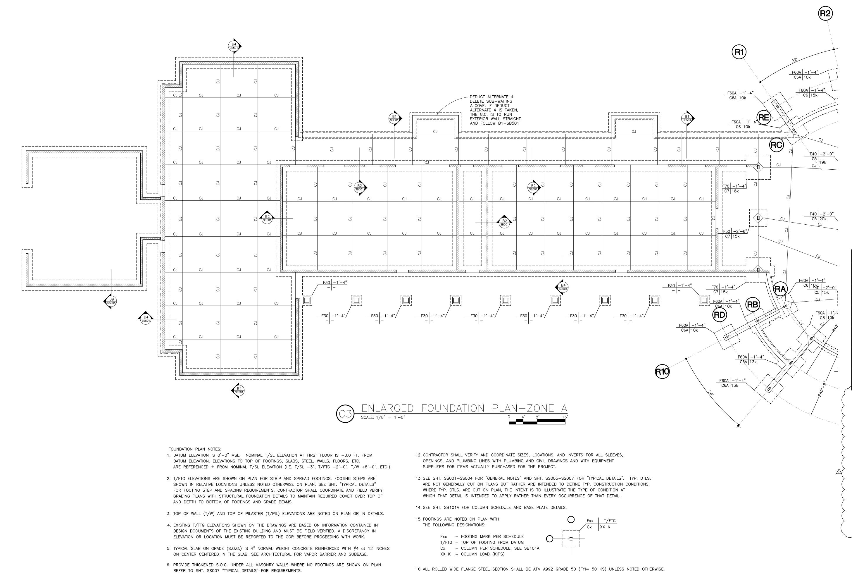
16. ALL ROLLED WIDE FLANGE STEEL SECTION SHALL BE ATM A992 GRADE 50 (FYI= 50 KS) UNLESS NOTED OTHERWISE. ALL OTHER ROLLED STEEL SECTIONS SHALL BE ATM A36 (FYI= 36 KS), U.N.O. EXCEPT HESS ROUND SECTIONS WHICH SHALL BE ATM A500 GRADE B (FYI= 46 KS) AND ATM A500 GRADE B (FYI= 42 KS) RESPECTIVELY.
