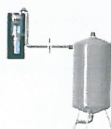
Hg5 installed remote from 50-Gallon Tank
