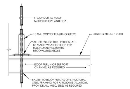
**3 CONDUIT ROOF PENETRATION DETAIL**
