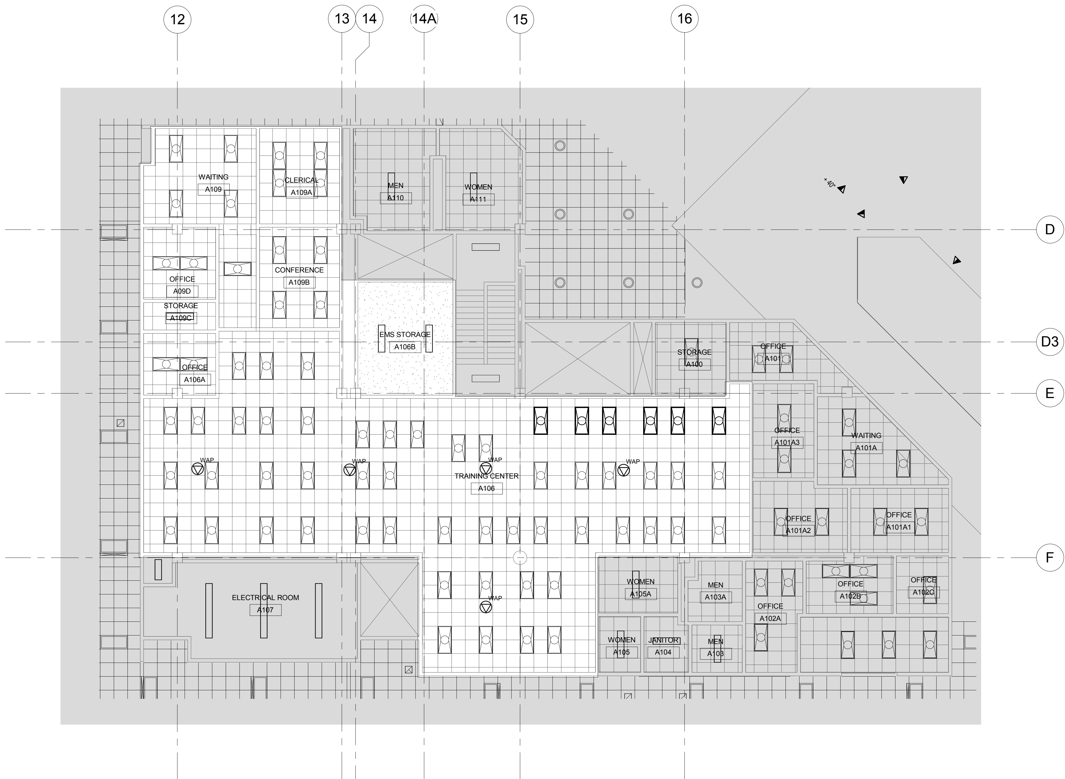
1 TELEDATA REFLECTIVE CEILING PLAN - BLDG 334 LEVEL 1 TRAINING CENTER CEILING PLAN 1/8" = 1'-0"
