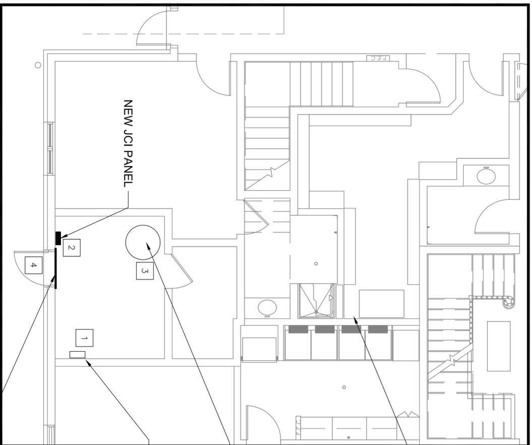
COMMUNICATIONS CLOSET. ROUTE NEW CONDUIT AND CABLING THROUGH BATHROOM INTO THIS LOCATION.
