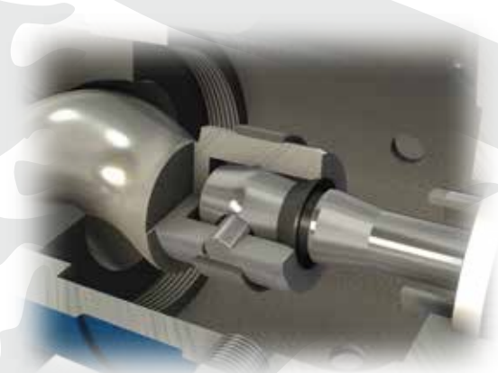
Cross Section of Pin Joint in the Rotor Head
