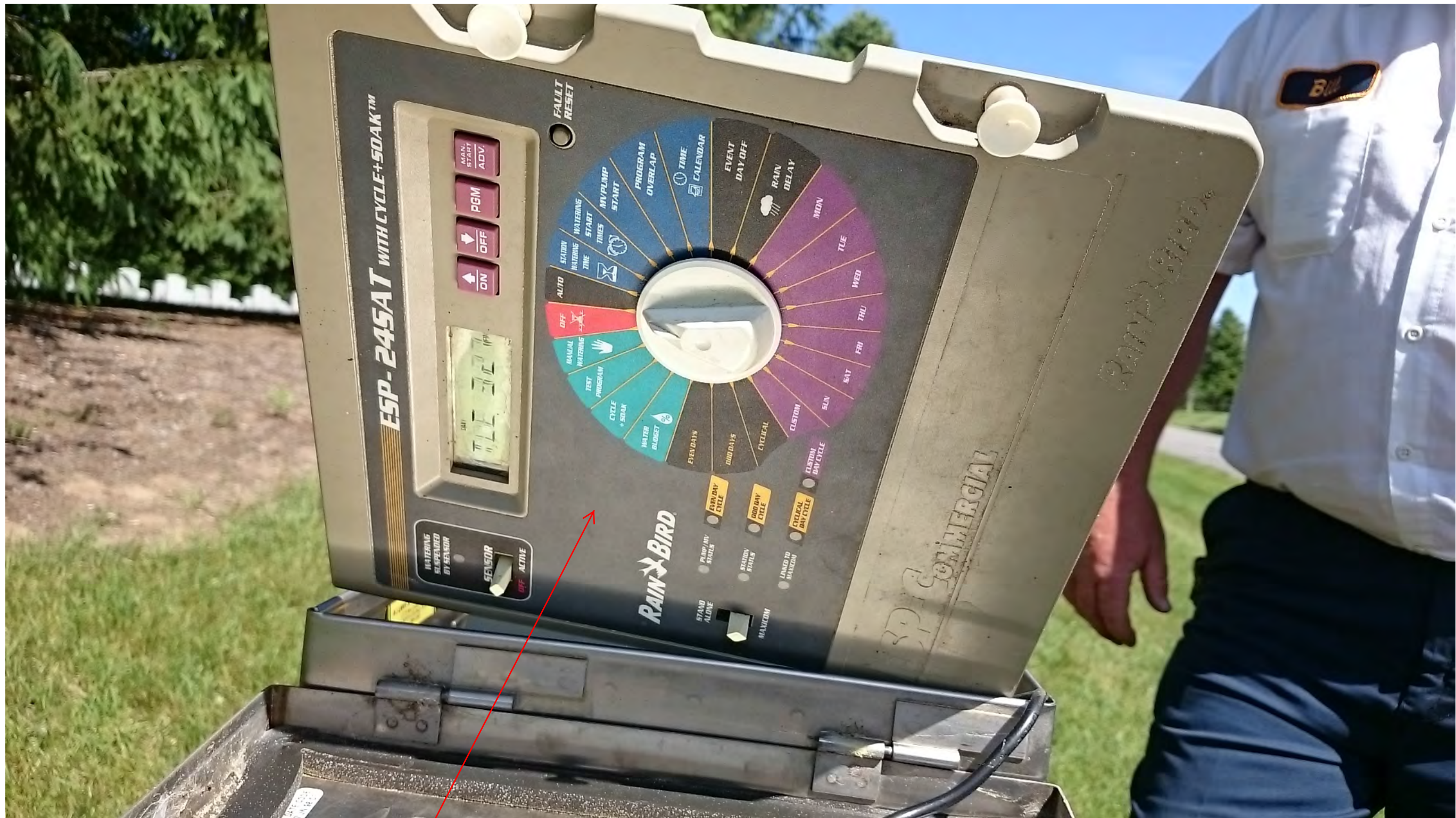
Details 2 and 3: Demolish existing graphical interface panel, circuitry, and all components including mainboard, antenna, and other electronics seen above. Install new to replace with a modern system and provide cemetery with a fully functional system.
