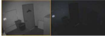
Illustra integrated PoE IR illuminators: shown in operation on the left, and when not in operation on the right.
