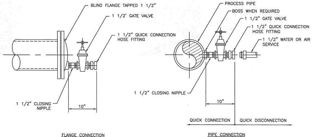
**PIPE FLUSHING CONNECTIONS**
