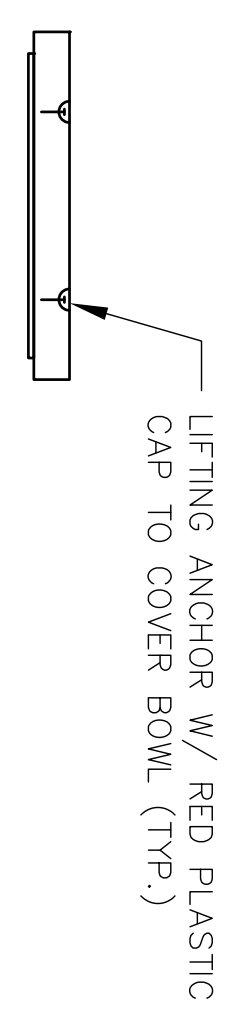
CRYPT LID - SECTION AT LIFTING ANCHOR NOT TO SCALE
