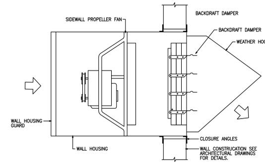
**SIDEWALL PROPELLER EXHAUST FAN DETAIL**
