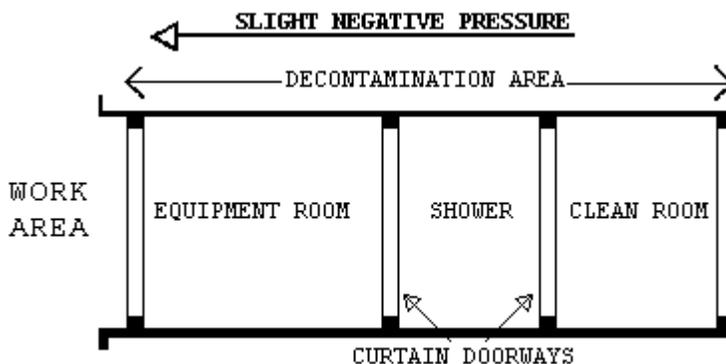
**1.9.5 WASTE/EQUIPMENT DECONTAMINATION FACILITY (W/EDF)**
