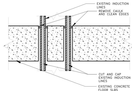
1 TYP. CONCRETE PIPING PATCH - UL263
