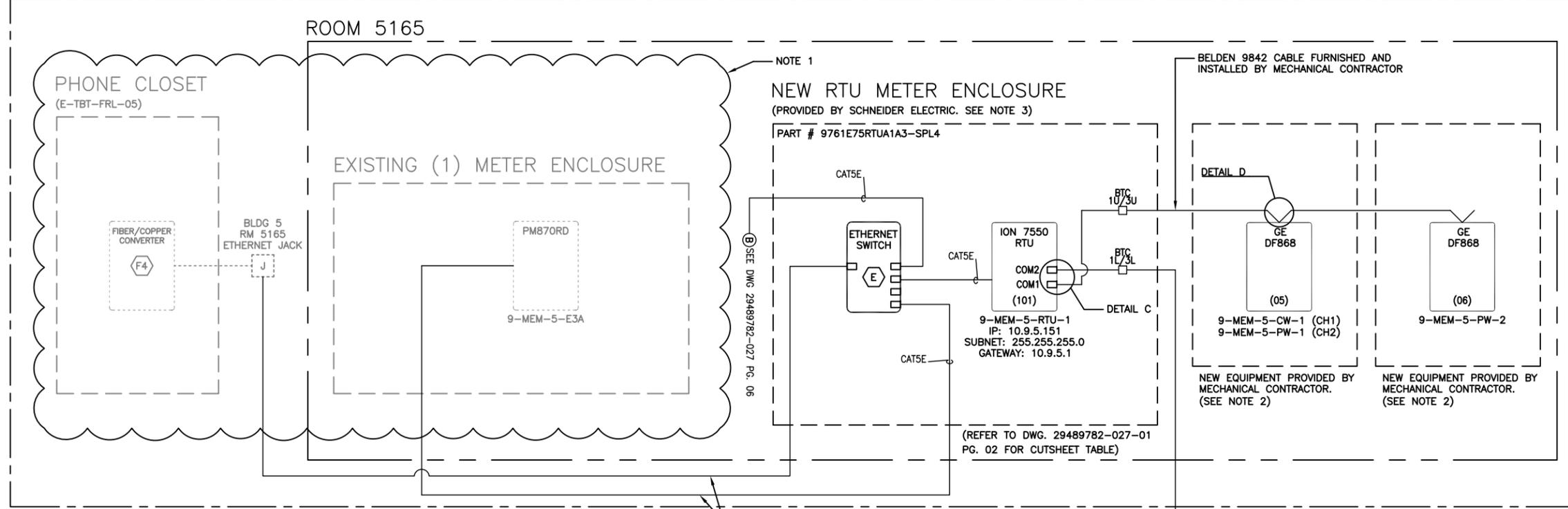
CAT5E CABLE FURNISHED AND INSTALLED BY MECHANICAL CONTRACTOR. FINAL EQUIPMENT CONNECTION TO THE EXISTING LAN TO BE MADE BY SCHNEIDER ELECTRIC FIELD ENGINEER.
