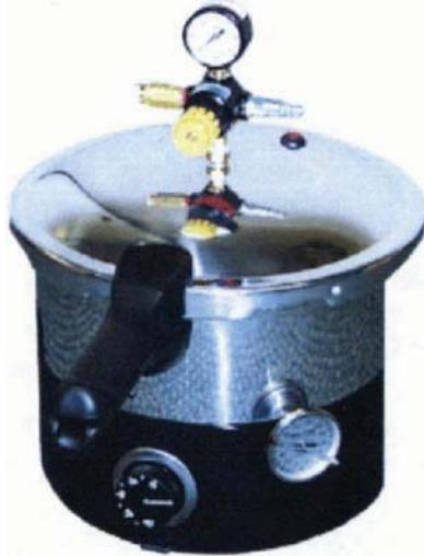
Used to cure a wide variety of acrylics requiring heat and pressure. Features a heat control thermostat and internal temperature gauge allowing for an accurate reading and setting of the internal temperature of the pot. The 6-quart pot has an internal diameter of 9.5 inches and depth of 4.75 inches. The 8-quart pot has an internal diameter of 9.5 inches and depth of 6.25 inches
