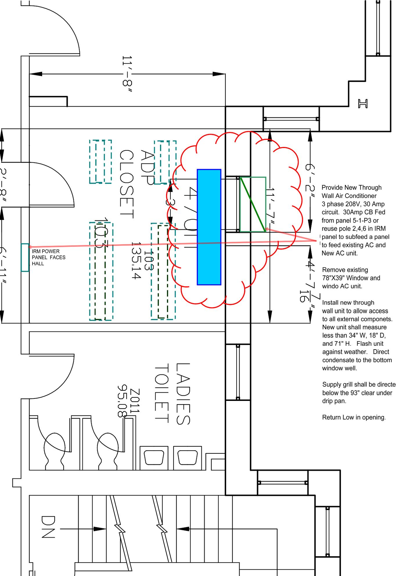
Provide New Through Wall Air Conditioner 3 phase 208V, 30 Amp circuit. 30Amp CB Fed from panel 5-1-P3 or reuse pole 2,4,6 in IRM panel to subfeed a panel to feed existing AC and New AC unit.
