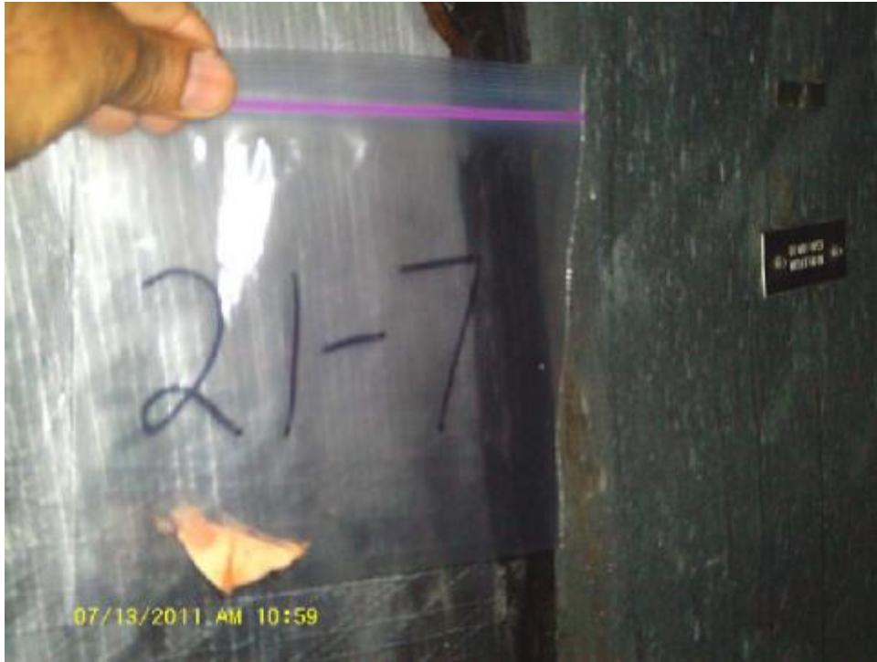
21-7 Black mastic on round duct insulation - AHU 21 3% Chrysotile in dark brown sealant
