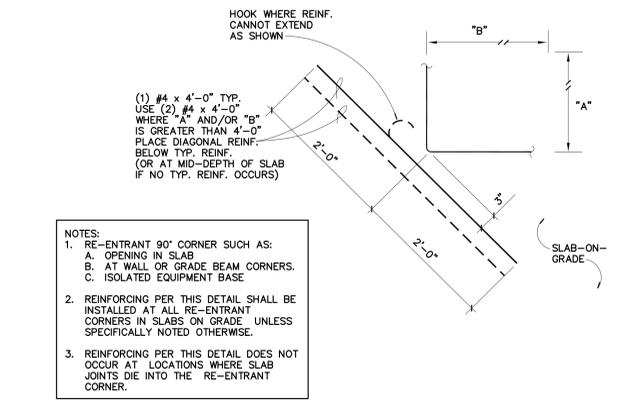
**REINFORCING AT RE-ENTRANT CORNERS IN SLAB**
