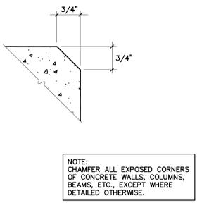
**TYPICAL CONCRETE CHAMFER**
