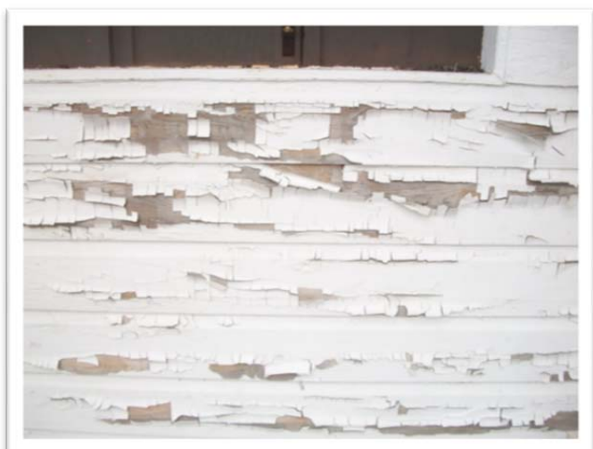
Sample 14-113A.L13, White Paint, 190,000 ppm Lead
