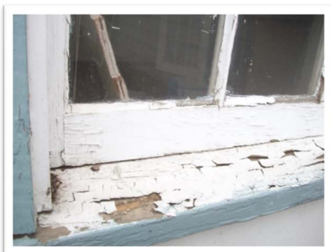
Sample 14-113A.L14, White Paint, 130,000 ppm Lead
