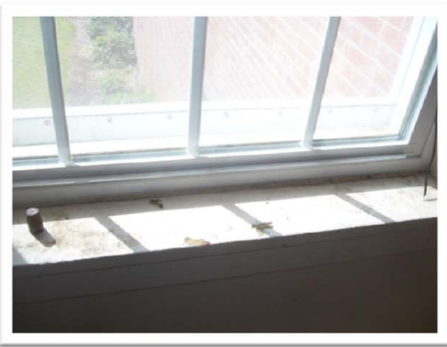
Sample 15-090A.L2, Window Sill, 1,400 ppm Lead
