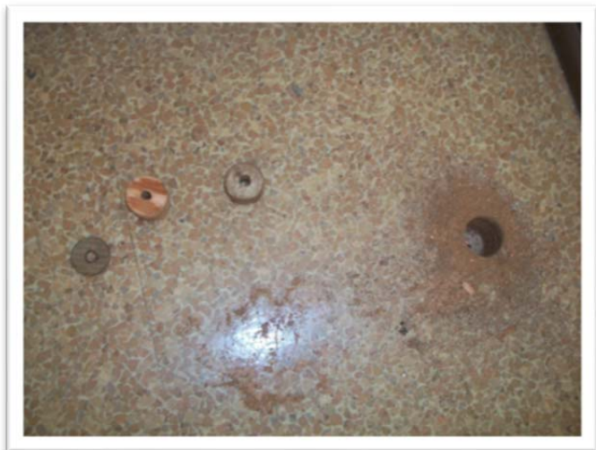
15-090A.21, Brown Vinyl Floor, 30% Asbestos 15-090A.22, Vapor Barrier, Non-ACM
