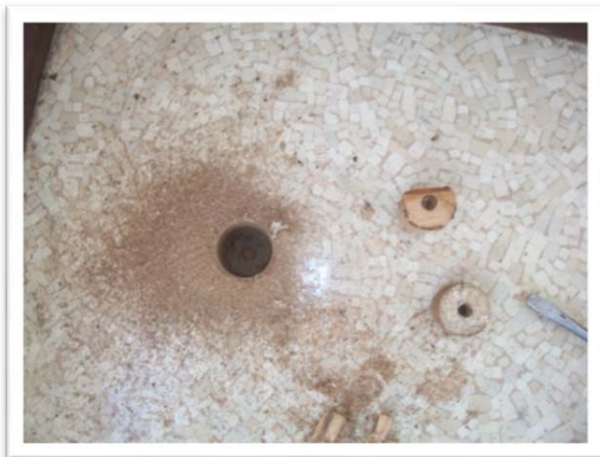
15-090A.23, Tan Vinyl Floor, 30% Asbestos
