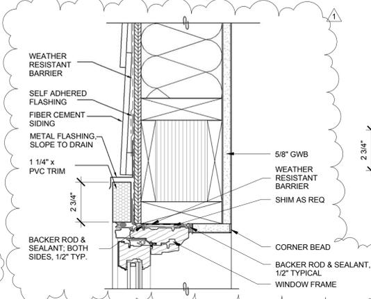
3 WINDOW HEAD AT FIBER CEMENT SIDING
